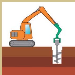
①先行掘削
